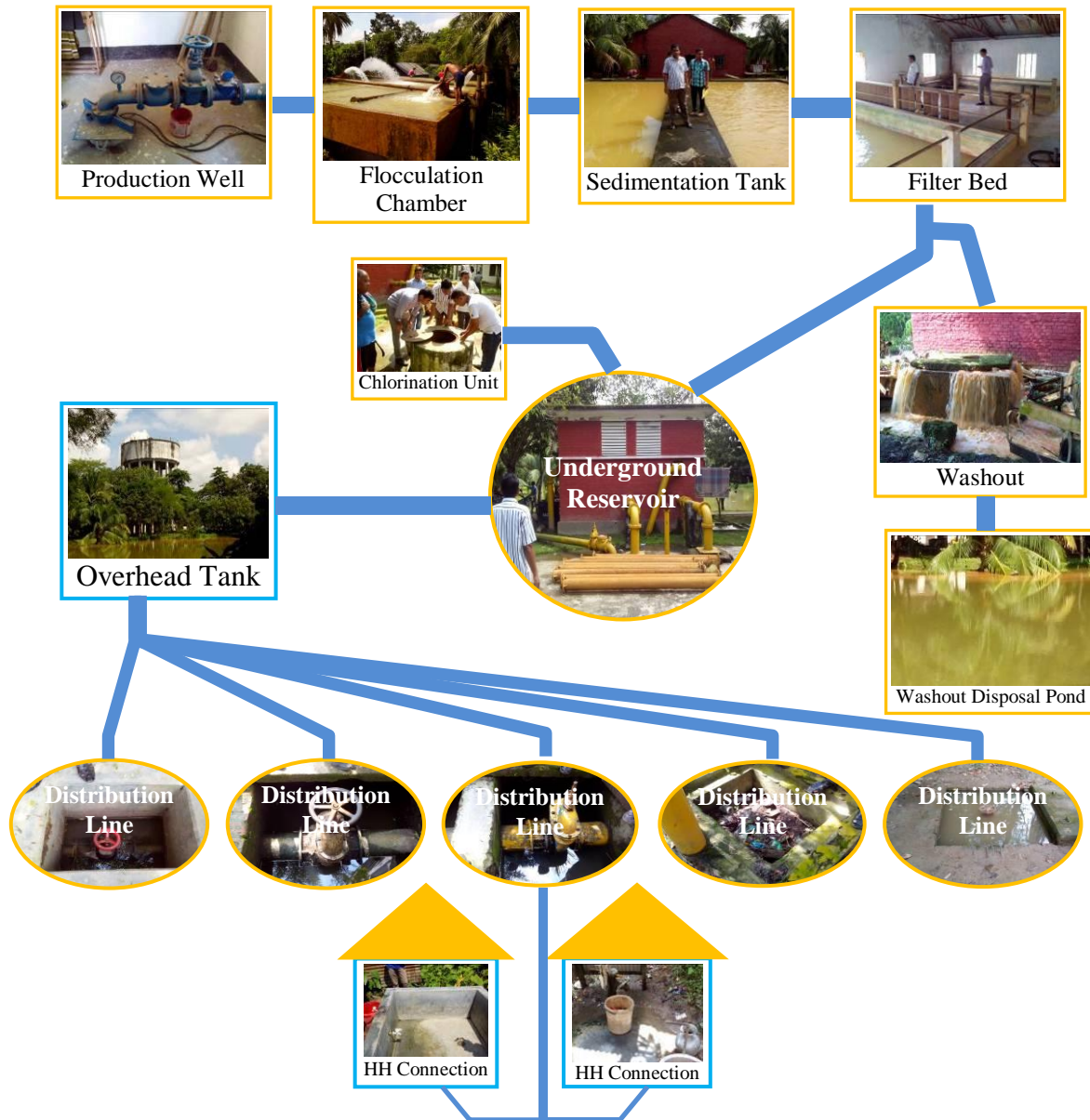
Fig. 1: Process flow diagram of the Faridpur Pourashava pipeline water supply system
