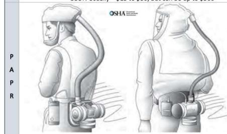
Loose-fitting powered air-purifying respirator (PAPR) Hood powered air-purifying respirator (PAPR)
