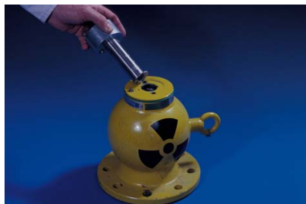
Lead radioactive source container with source holder removed (HPA)
