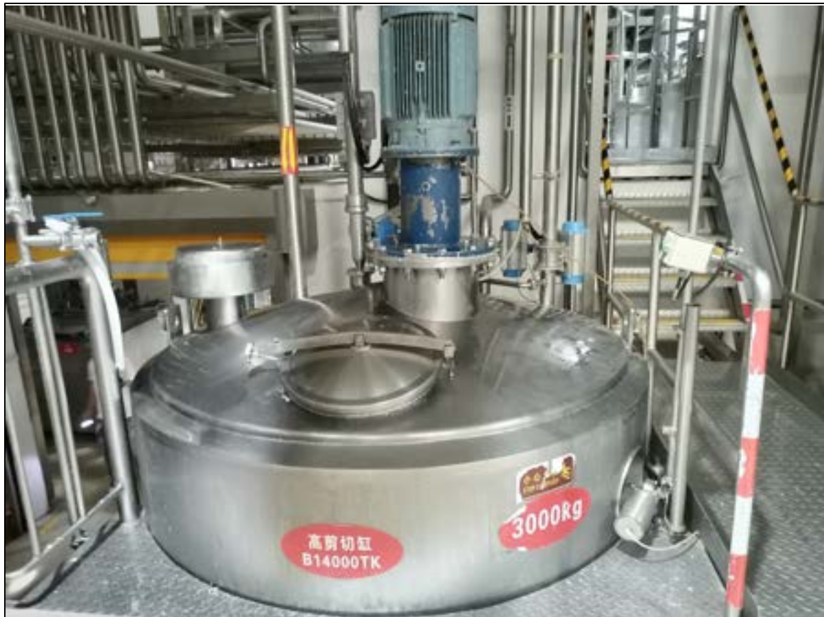
Figure 12. Top view of mixing tank and dosing area for powders and pastes containing food allergens
