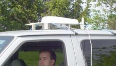
A low-cost, fully integrated and portable system for mapping RF fields or power density around mobile phone base stations (developed by Health Canada's scientists).
