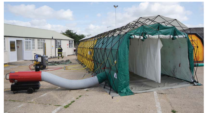
Figure G2. Example of a specialist mass decontamination unit. Photo: HPA.
