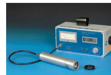
Figure A8.10. Examples of NaI(Tl) detector based monitors used as gamma contamination monitors. Photos: HPA.
