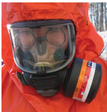
Figure A2.1. Full face mask and filters are the basic respiratory protection for CBRN units. A correctly fitted full face mask should not have an inward leakage above 0.05 %. Filters are classified into P1, P2 and P3 classes with filter penetration less than 20 %, 6 % and 0.05 %, respectively. Class P3 filters should be used with full face masks to obtain the best protection factor. Photo: STUK.
