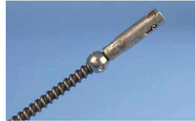
Figure E5. Very dangerous source from radiography camera (should never be picked up). Photo: HPA.
