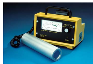
Figure A8.10. Examples of NaI(Tl) detector based monitors used as gamma contamination monitors. Photos: HPA.
