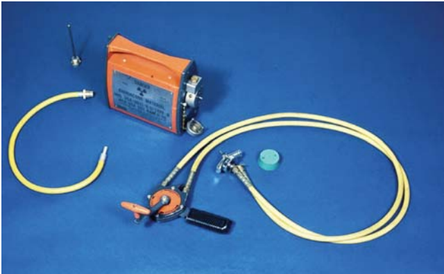
Figure E4. Typical radiography camera. Photo: HPA.
