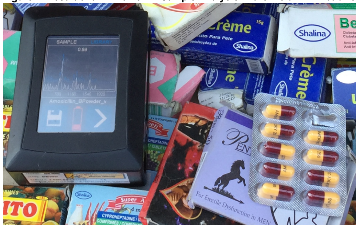
Figure 4. Result of an Amoxicillin Sample Analysis in the Field in Zimbabwe
