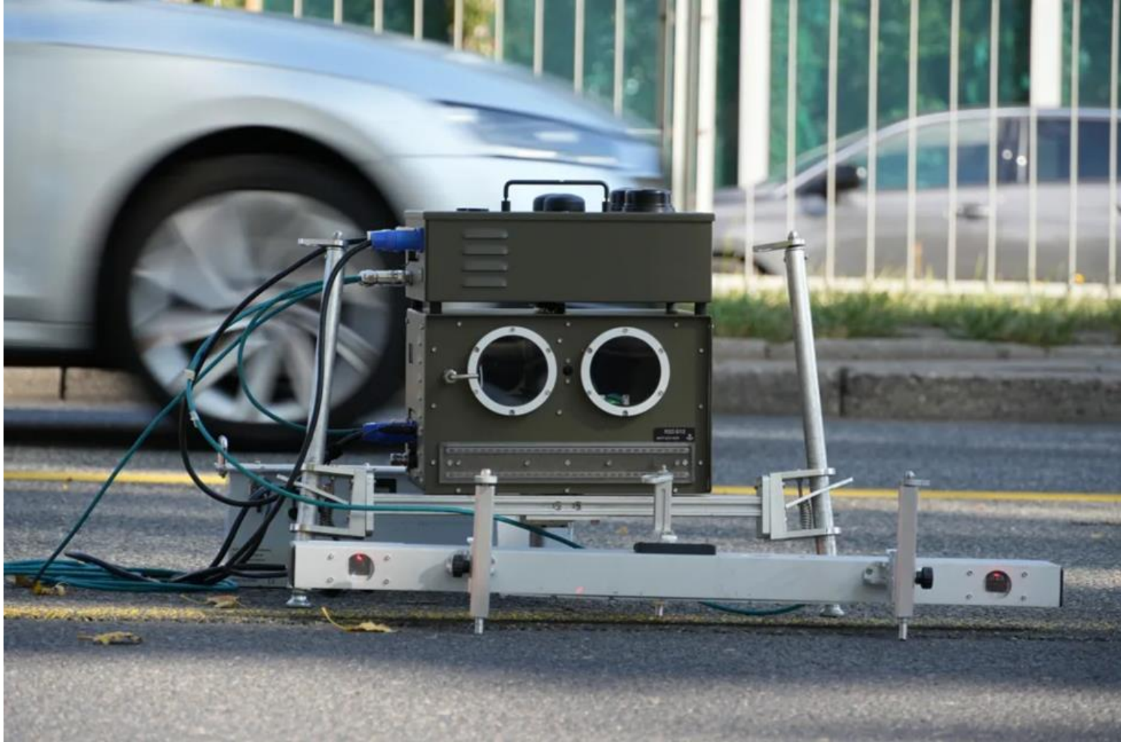
Roadside testing equipment measuring real-world emissions. Warsaw, Poland. 2025.
