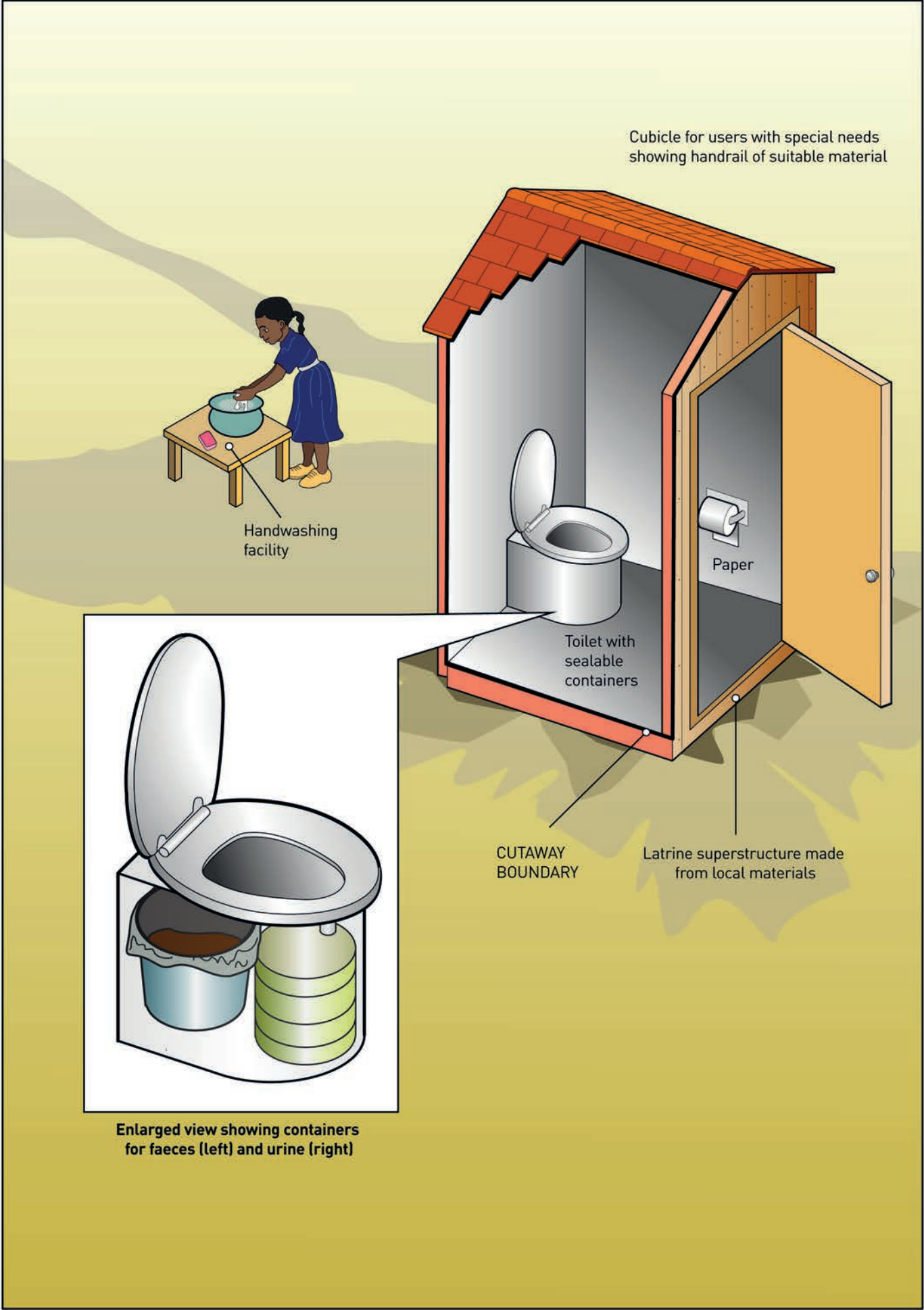
Urine diversion dry toilet with cartridges or storage tanks
