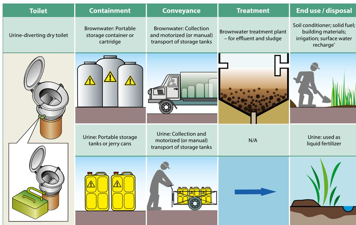
\* Sludge: treated and used as soil conditioner, solid fuel or building materials. Effluent: treated and used for irrigation or surface water recharge.
