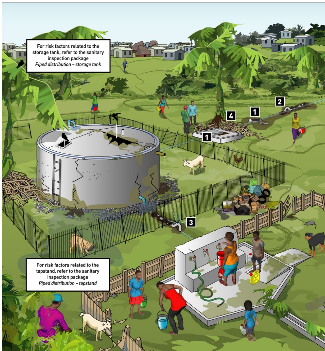
Figure 1. Typical risk factors associated with a piped distribution network
